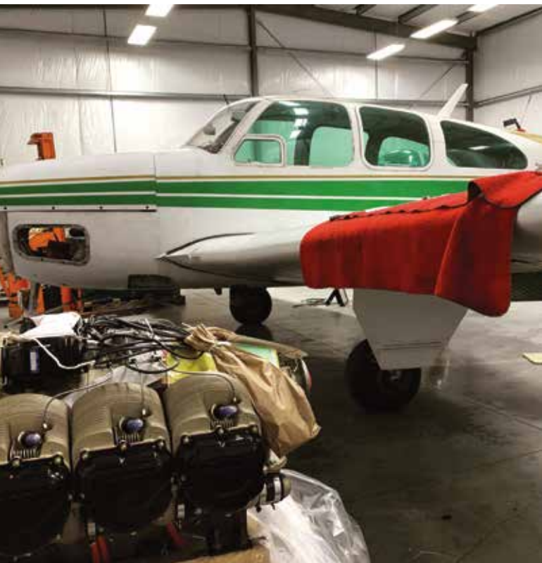
Original configuration. Starting installation of a new IO-550B.
